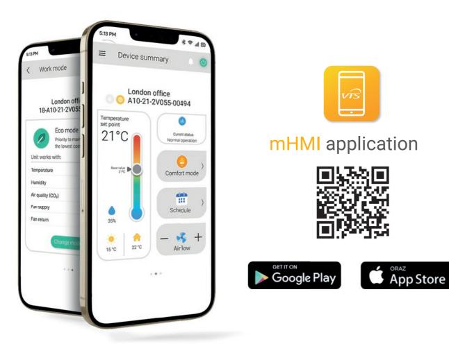
The app connects to the unit using Bluetooth technology. All you need to do is launch the app and activate the Bluetooth module, which is located in the automatic control cabinet. The app will automatically detect the unit which you can then connect to.
